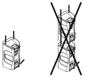
Figure 4.5: Loudspeaker vertical suspension (Correct, left; Incorrect, right)
