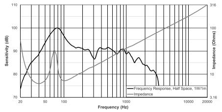
Figure 7.10: ELX200-18S frequency response and impedance
