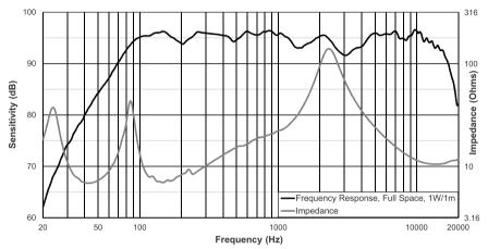
Figure 7.8: ELX200-15 frequency response and impedance
