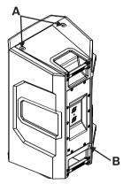
Figure 4.1: Suspension points (A top, B bottom)
