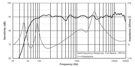
Figure 7.6: ELX200-10 frequency response and impedance
