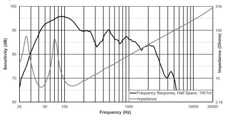
Figure 7.9: ELX200-12S frequency response and impedance
