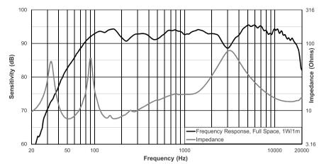
Figure 7.7: ELX200-12 frequency response and impedance
