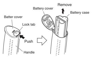
Step 2. Insert six AA batteries referring to the polarity diagram on the inside of the battery compartment.
