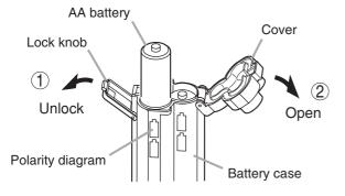
Step 3. After confirming the correct battery polarity, close the battery case cover. Ensure that the cover is securely locked in place with the lock knob.
