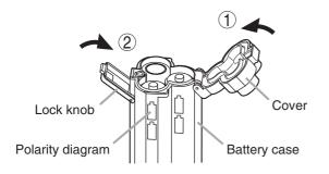
Step 4. Replace the battery case in the handle and close the battery cover.
